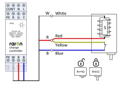
There can be different colour wires used for DSIEC-EL solenoids, therefore it is advised to consult the datasheet of the manufacturer. The connections can also be determined using a multimeter.
