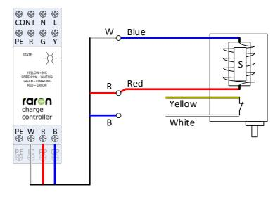
There can be different colour wires used for DSIEC-ELC solenoids, therefore it is advised to consult the datasheet of the manufacturer. The connections can also be determined using a multimeter.
